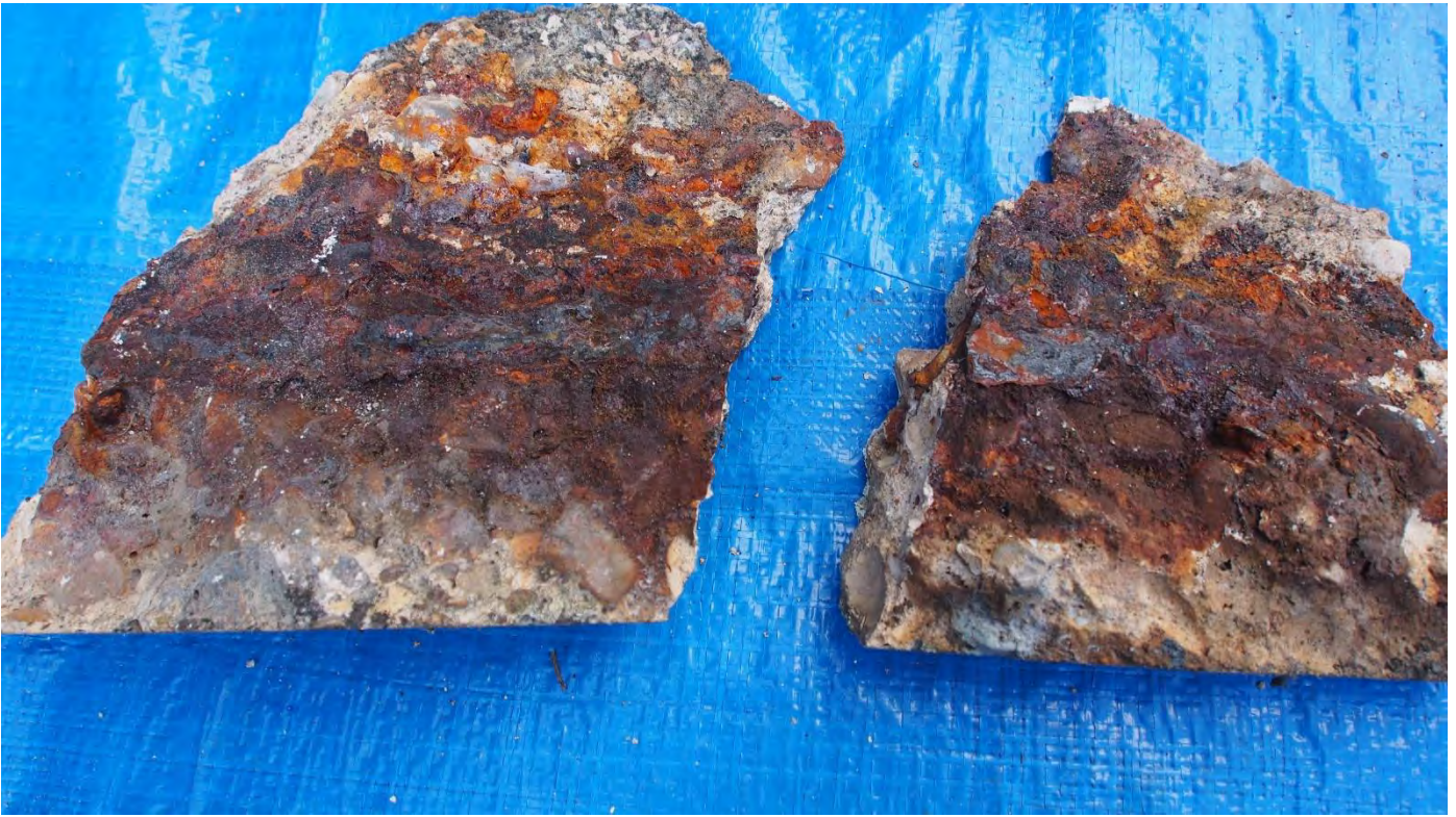
Typical Removed Section of Balcony Panel Bottom Drip Detail found loose and painted over Loosened due to steel bar corrosion
