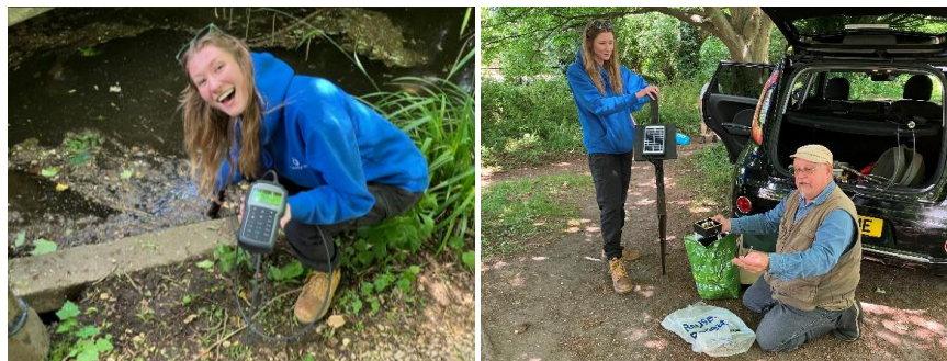
Left: Sarah, Cambridge Water testing Hanna HI-98594 multiparameter probe to monitor turbidity, temperature, electrical conductivity, pH and dissolved oxygen. Right: Dr Steve Boreham demonstrates a ThinkSpeak-enabled data logger.
