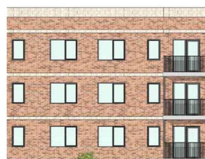
2. Constructing protruding brickwork banding at each level creates a horizontal emphasis. Stacking the glazing vertically gives the facade rhythm.
