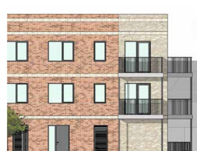
4. Changing the colour of the brickwork on the corner of the building highlights the edge condition and defines the vertical stacking of the balconies.
