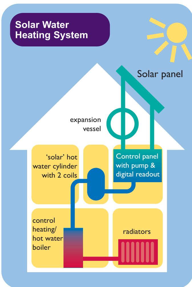
the summer, and even in winter on a cloudy day could still provide up to 20% of the heat required for hot water. Current installation costs are around £3,000 per system (£1,500 if installed by DIY) but this is likely to decrease over time.
